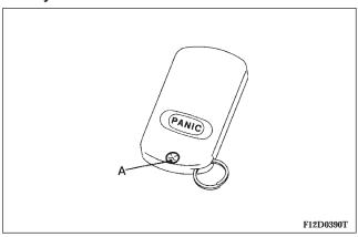
1. Remove the transmitter case mounting screw (A) and gently pry open the case.
